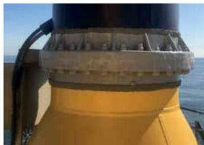
An offshore crane flange protected with the Oxifree coating solution
