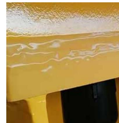
A close-up shot of an Easy-Qote corrosion-preventative patch
